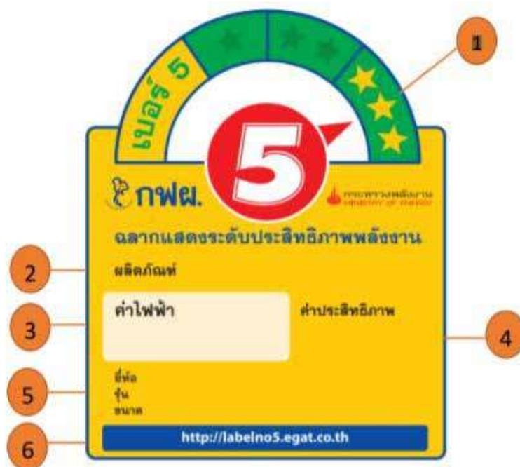
Figure 1.2: Thailand energy efficiency no.5 label (1: Energy efficiency level, the highest efficiency is 3 stars, 2: Indicates the type of product that has been certified, 3: Electricity bill per year to compare and estimate electricity usage, 4: Performance value for comparison with other products of similar size, 5: Product information, including brand, name, model, size, to be able to check the preliminary, 6: website of the Electricity Saving Label Project No. 5) (Source: Sustainable Consumption and Production Baseline Research for ASEAN, 2019)
